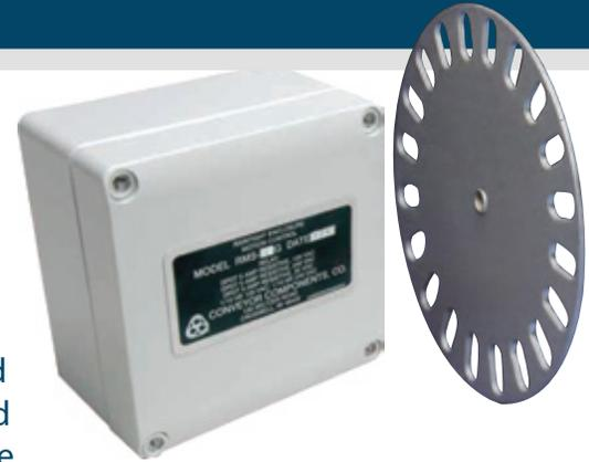
The Model RMS uses a remote mounted inductive sensor to monitor speed. Motion is sensed by means of induced measurable pulses produced by a ferrous metal target rotating past the sensor. If a distinctive metal target is not available an optional metal disk can be purchased. The produced pulses are converted to a digital electronic signal. Solid state circuitry within the DIN rail mount box then analyzes the digital signal and activates or deactivates the output relay at the pre-set speed point.
