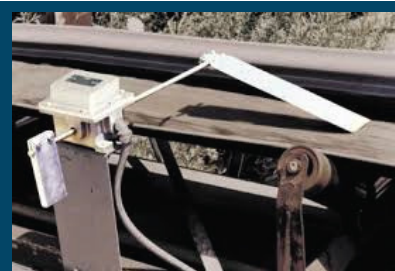
FS Flow Switch is in position to indicate any interruption in the flow of material along the last moving conveyor belt.
